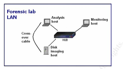
Physically and logically the lab LAN was isolated, or air-gapped, from any other systems. There were no physical (cable) connections from any of these devices to any other network or communications system. The lab LAN was setup in a low traffic, locked room and all systems were powered down when not actively involved in the analysis process.
